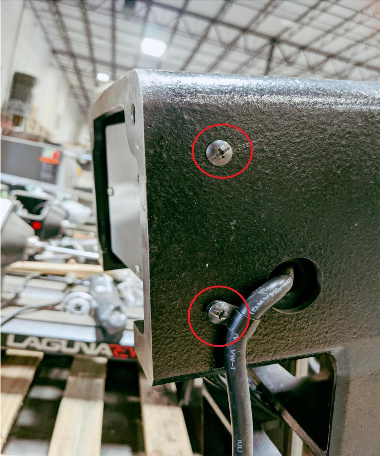
3. Remove wiring as shown (*we recommend loosening and re-connecting one at a time*). Remove and replace board. Do steps in reverse order to put machine back together. **It is CRITICAL that wired connections are reconnected to match the original board orientation.**
