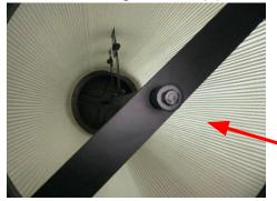
Open the canister filter doors and secure the HEPA canister filter onto the dust chute by fastening the band clamp on the top part of the HEPA canister filter. Make sure the band clamp is tightly fastened. It does not matter which side the clamp faces.
