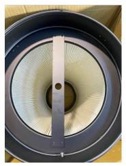
Turn the HEPA filter right side up and insert the filter rotation shaft assembly into the HEPA filter from the top opening. It will be easier to insert while holding it at a slanted angle. The rotation shaft has a top and bottom end. The top end has bolt holes for the next step. The bottom of the shaft will fit into the rotation shaft base at the bottom of the filter.
