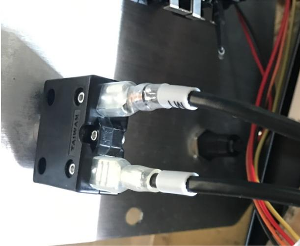
8. Loosen the bolt holding the onboard overload button using a wrench.
