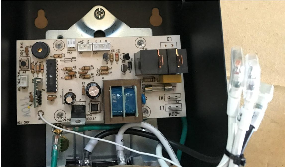
5. Carefully and gently loosen the four plastic bolts on the circuit board and set aside for use in the next step. Remove the 110v circuit board and replace with the 220v circuit board. Make sure the direction of the 220V circuit board is attached in the same position as the photo shown below.
