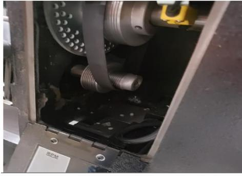
5. Using a 3mm Allen wrench, remove handwheel (*casing*) by loosening 2 small screws that are oriented opposite each other.
