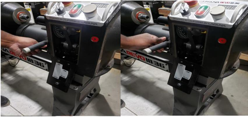
3. Lift up on motor adjustment handle to lift motor up to physically lift motor into a position where the belt will loosen.
