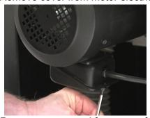
5. Remove power cord from rear of saw by removing 2 screws in retainer plate.
