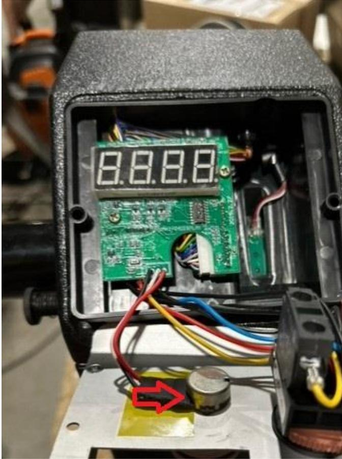
After removing all these pieces, you should be able to pull the DRO completely out. The next step would be to install the new DRO the same way you took the old one off.
