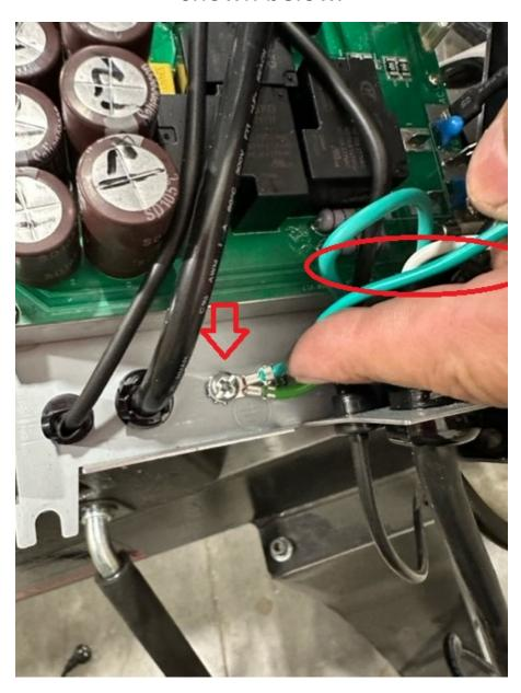
Step 3. Remove the wire bracket shown in the picture below.
