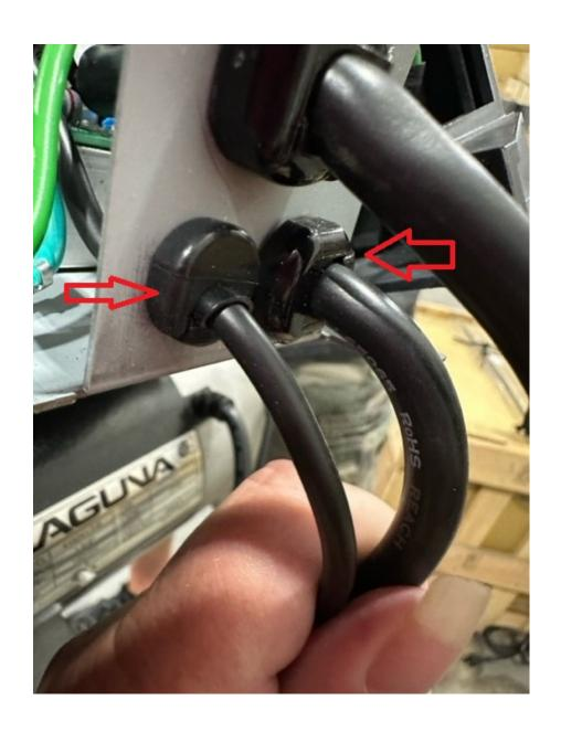
Step 5 and 6. After the wires are removed, you will then move to the front of the headstock and remove the belt
