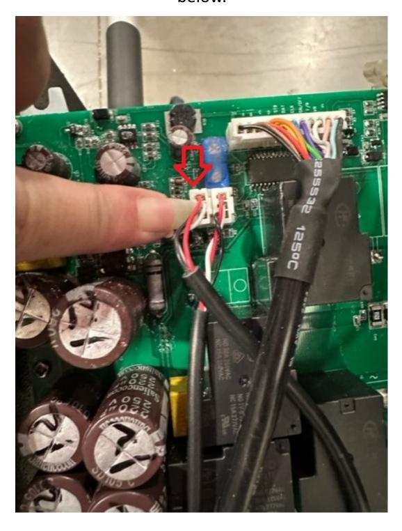
Step 4. Remove the strain reliefs by squeezing with pliers, turning 90 degrees and pulling the wires out.
