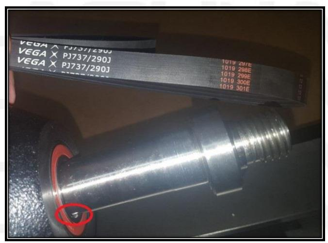
Note: If the inboard bearing comes out with the spindle, this is fine. Just proceed with the steps as normal. This will make some of the following steps considerably easier. You will just need to dislodge the bearing to insert it into the headstock before inserting the new spindle.
