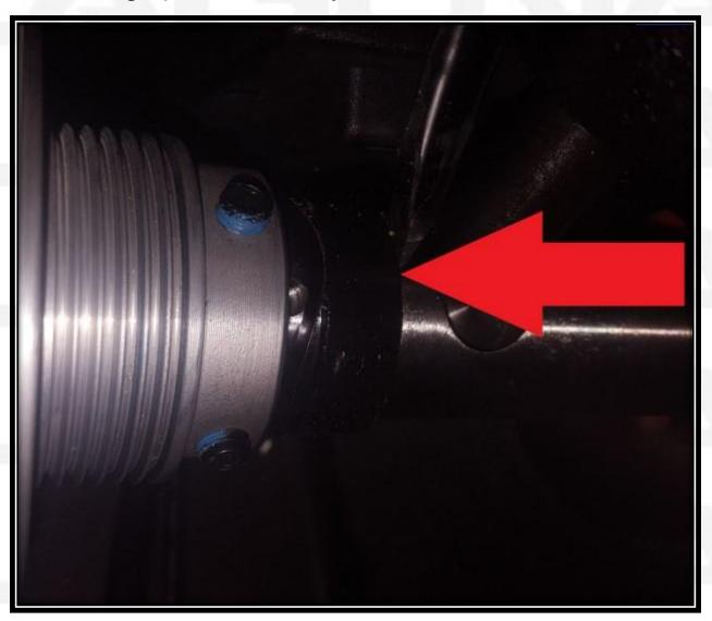
Once this is free to move, you can slide it and the pulley off the left side of the spindle while pulling the spindle out of the inboards (Right) side of the headstock and everything is disassembled!
